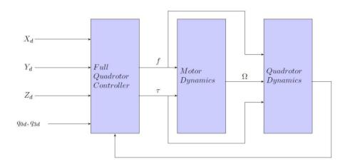
Figure 2. One Loop Control Block Diagram.
