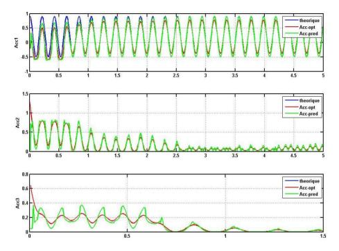
Figure 6. Estimation and prediction of the acceleration of the end effector.
