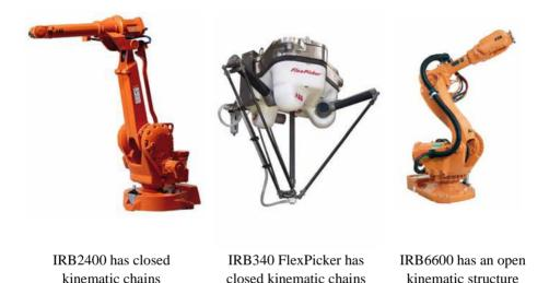
Figure 2. Robot configurations found among the ABB robots.
