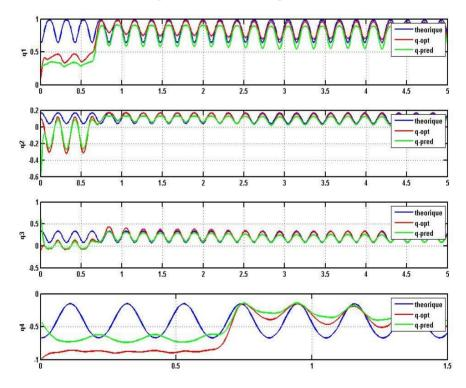
Figure 5. Estimation and prediction of the quaternion for the end effector.
